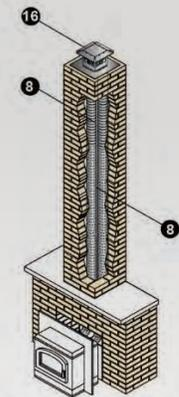
Co-Linear SS Flex Installation for Pellet Inserts
